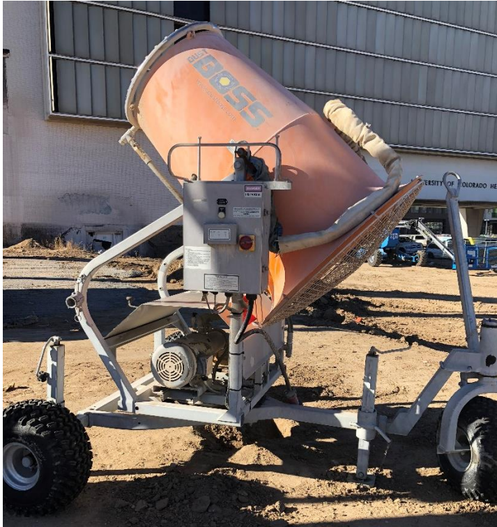
Photo 3: Dust Boss Dust Control Unit
